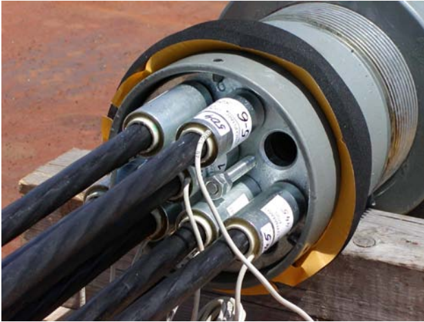
Fig. 1. Assembly of PSS22 sensors
